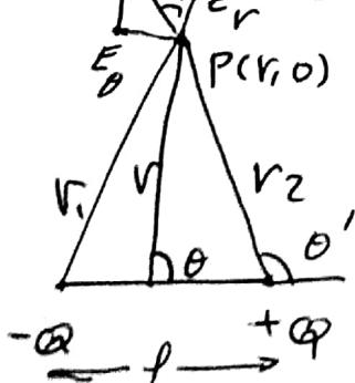
$$(1) \Phi = \frac{Q P (l + 2r_2 \cos \theta')}{4\pi \epsilon_0 r_1 r_2 (r_1 + r_2)}$$
