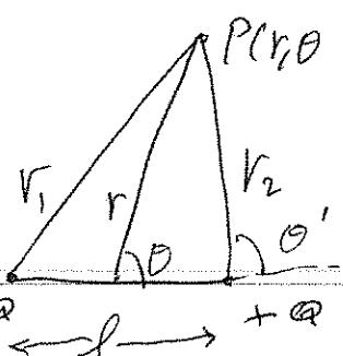
$$② \phi = \frac{1}{4\pi\epsilon_0} \frac{Q}{r_2} - \frac{1}{4\pi\epsilon_0} \frac{Q}{r_1} = \frac{Q(r_1 - r_2)}{4\pi\epsilon_0 r_1 r_2} \quad (1)$$
