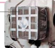
This air scrubber used lithium hydroxide to purify the air inside the Apollo 13 spacecraft
